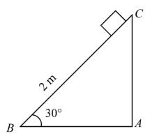
A block of mass 2 kg from vest slides down an inclined plane of length 2m, inclined at an angle of 30°. Its kinetic energy at the bottom is 15.6 J.
